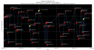
Figure 2: Diary of satellite 1126 in the Starlink constellation between 2021-02-12 and 2021-02-17
